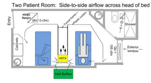
**Figure 2.** Example schematic of a two-patient expedient patient isolation room configuration. In this configuration, the occupied inner isolation zone shows the make-up air gap and HEPA filter exhaust inlet positioned to induce directed airflow across the head of patient's bed. A pvc-framed tunnel was erected near the HEPA outlet to facilitate HEPA exhaust discharge without disrupting plastic curtains.
